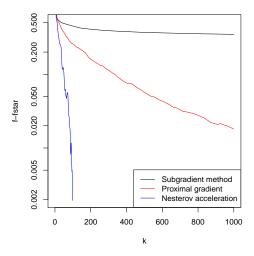
Note: accelerated proximal gradient is not a descent method
